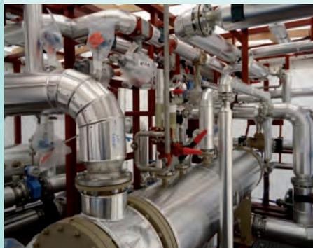
⤴ In the prototype, heat exchangers are 3 or 4 meters long. On a real scale, they reach a 12 meter length and a 4 meters diameter.
